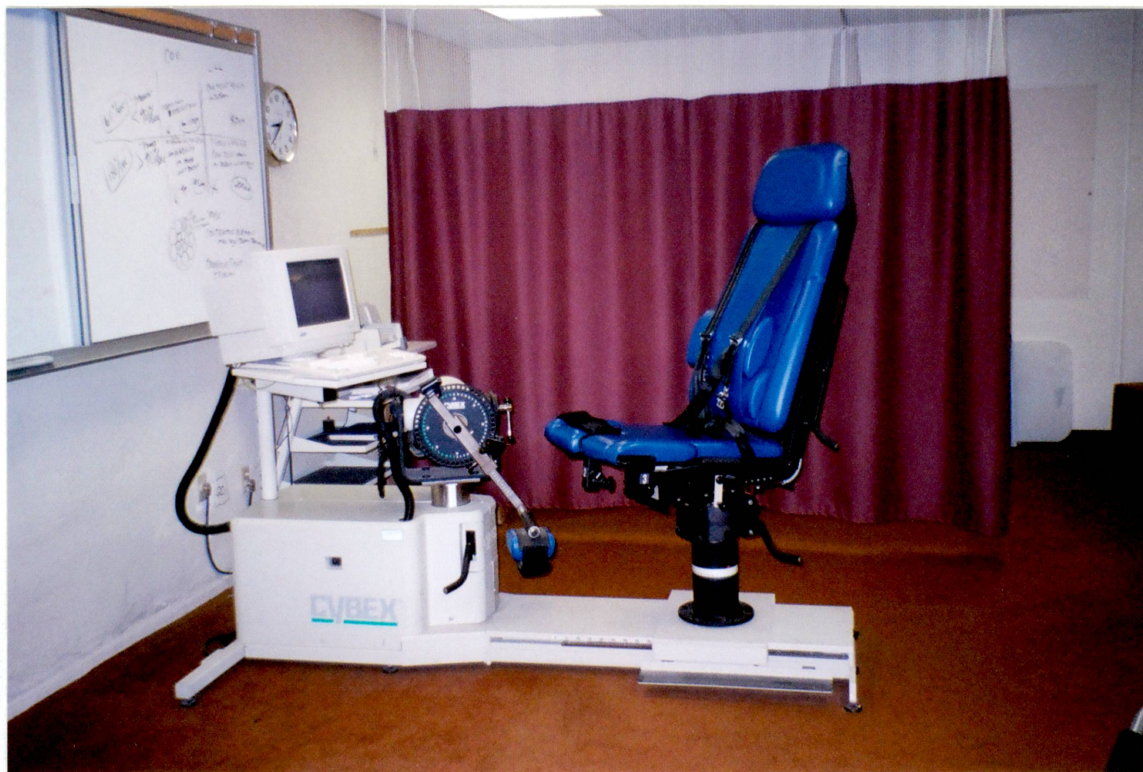
Figure 1. Cybex Norm Isokinetic Dynamometer parts and components.
